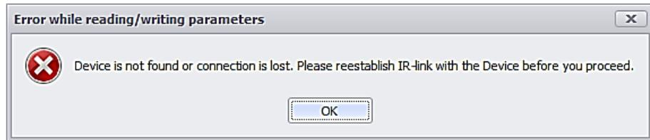
In this case re-establish IR-connection between the instrument and PC and try reading/writing settings again.
